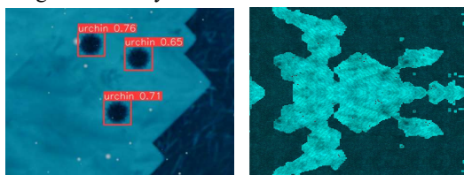
Fig 2. Left: Inference examples of the trained yolov8n network during the online execution in the Stonefish simulation. The generated bounding boxes along with their confidence score are displayed. Right: Simulation environments mimicking a seabed containing sand, Posidonia oceanica and sea urchins.
