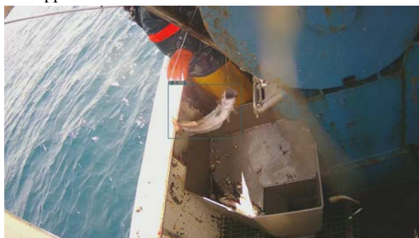
Figure 1. Snapshot that shows the detection of a specimen in a frame of a captured video, the trained network locates the specimen area with a detection rectangle. It associates a prediction about the calibre and a score. In this case, calibre 3 with a score of 0.69.
