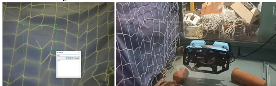
Fig 1. At the left the net hole labeling and at the right the BlueROV2 inspecting the net
