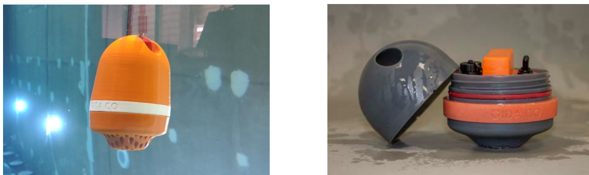
Fig 1. A: FDM prototype immersed in water. B: SLA prototype open.
