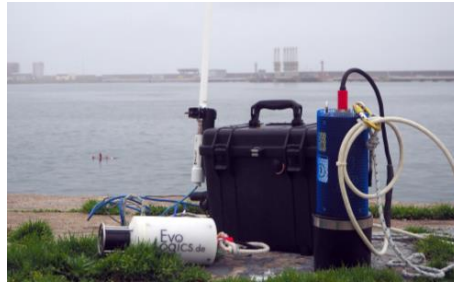
Fig 1. Manta gateway with two distinct acoustic modems
