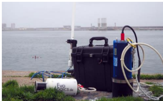
Fig 1. Manta gateway with two distinct acoustic modems
