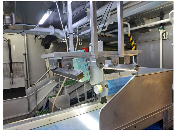
Fig 1. iObservers 2.0 installed on board R/V Miguel Oliver
