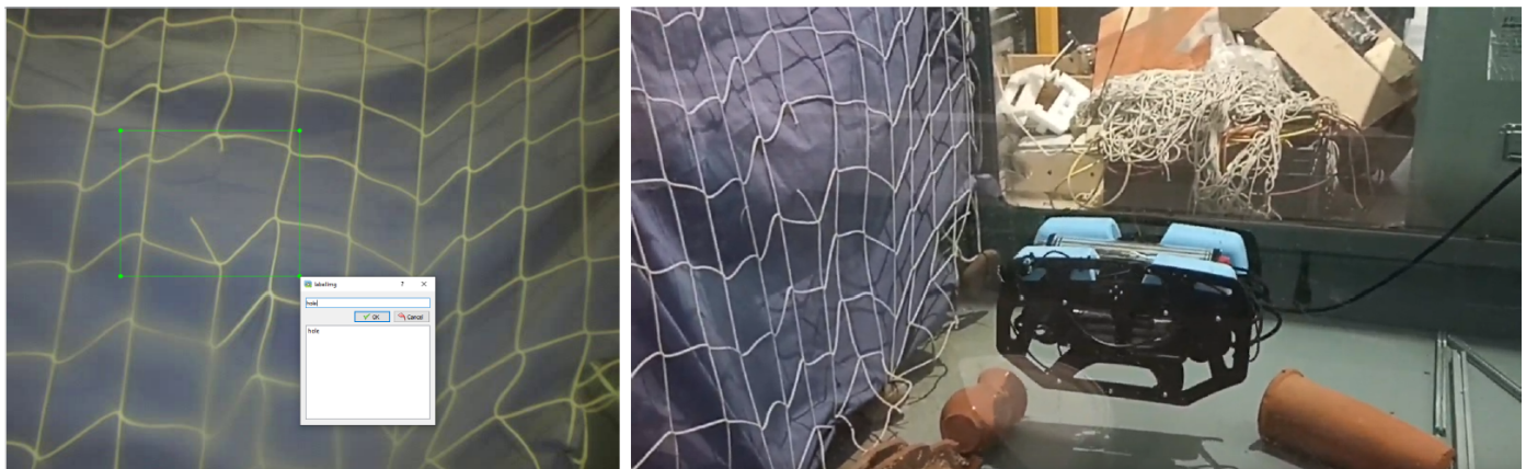
Fig 1. At the left the net hole labeling and at the right the BlueROV2 inspecting the net
