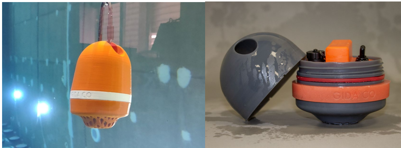
Fig 1. A: FDM prototype immersed in water. B: SLA prototype open.
