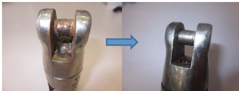
Illustration 2. Electrolytic cleaning was also applied to pieces of boats of the Spanish Naval Academy.
