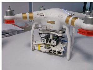
Fig 1. Payload mounted on a DJI (Phantom IV) quadcopter. Housing can bear one or two cameras.
