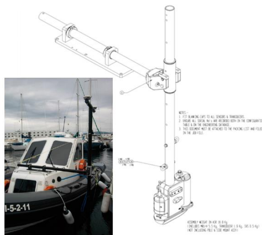
Fig. 4. Blue print and view of the structure in full swing pole, installed in the INNDAGA boat to anchor the multibeam system plus GeoSwath of Geoacustics and GPS antennas on line.
