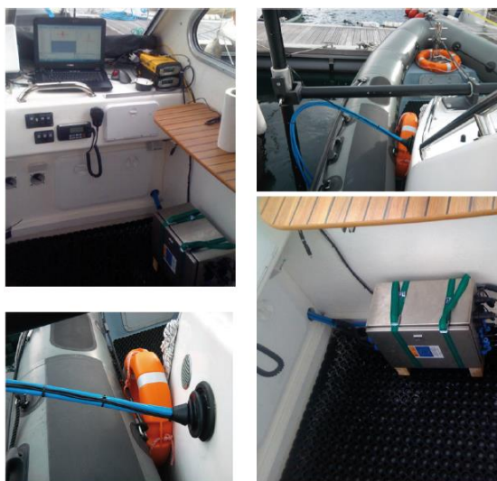
Fig. 3. Detail of the installation of the operating unit within the cabin under the folding table and the top right are seen the GPS in yellow. The solution adopted is also shown for output cables to the transceiver unit in the two photographs bottom of the figure.
