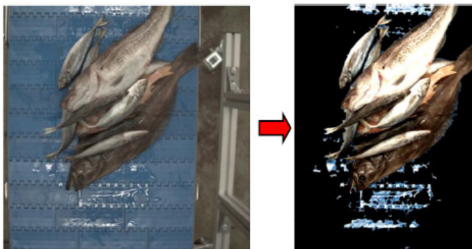
Fig. 3. Image background (conveyor belt) removing.
