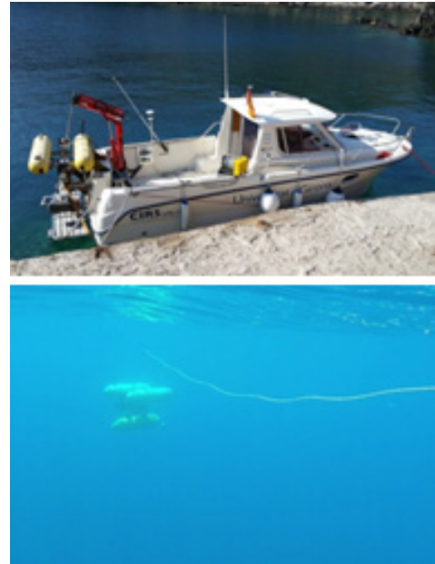
Fig 2. Girona 500 HROV ready for the experiment on top of a 7 meters boat having the USBL positioning system and the electrical winch for the umbilical communications (top). The HROV has a light 30 meter umbilical cable, which allows a free movement of the vehicle, connected to a vertical 200 meter metallic cable which is provided by the winch. The boat maintains its position on top of the HROV by using the estimates of the USBL.
