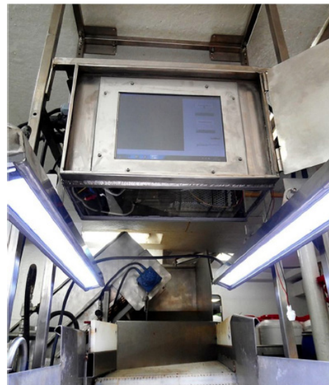
Fig. 1. Main Box and external lighting as they were mounted in the oceanographic vessel: Vizconde de Eza.
