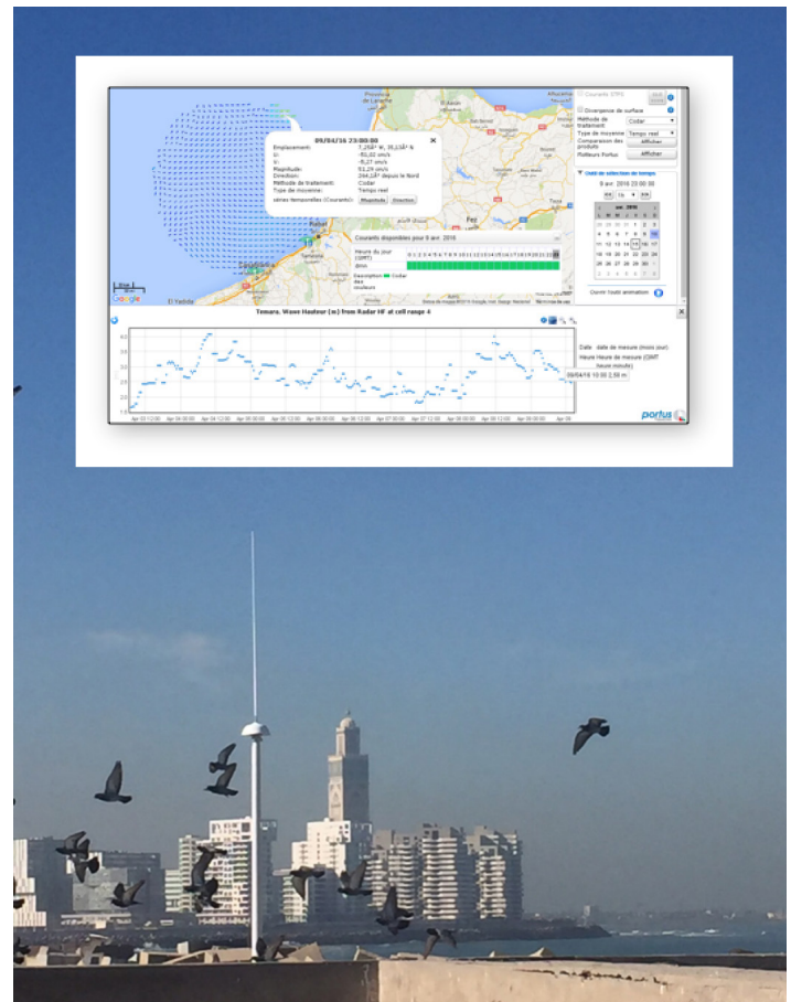
Fig. 6 Compact 2 x 4.5 MHz SeaSonde HF Radar system in Morocco and principal 2D deliverables, currents mapping and waves monitoring. (HF Radar system operated by the Direction de la Météorologie Nationale).
