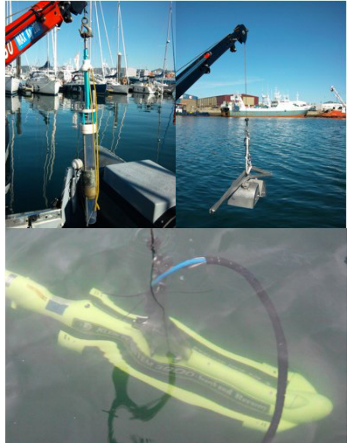
Fig 5. Piston corer and van Veen grabber being deployed.
