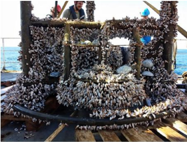
Fig. 4: cirripods on BOREL's keel after recovery in 2015
