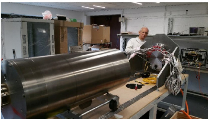
Fig 1. Above: Construction of the Cable End Equipment (CEE).
