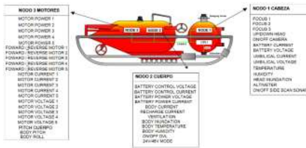
Fig 3. The UUV (left). CANopen network distribution.
