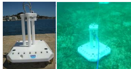
Fig. 2. Underwater Sensor Units (USU) of the Multi-Influence Range System, MIRS.
