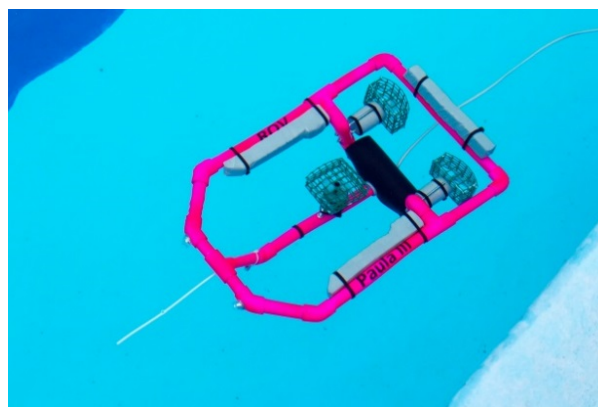
Fig. 1. Own production ROV (without accessories)
