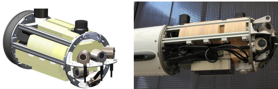
Figure 4. Design and picture of a complete sonar and video payload.
