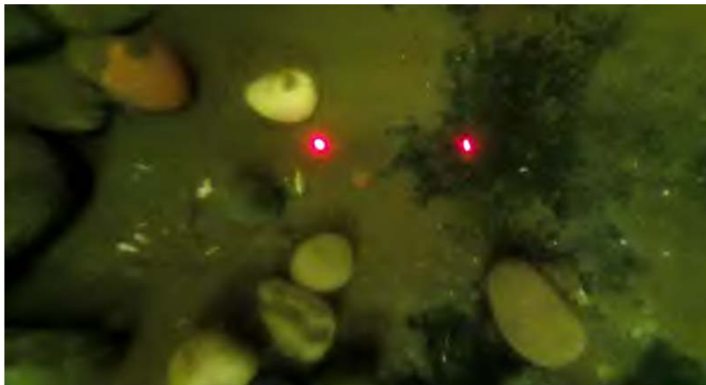
Fig. 2: Image compression experiments conducted at IRSLab-UJI laboratory in water tank conditions. Images with a resolution of 1200x650 pixels have been compressed and transmitted through a 868Mhz radio channel at 1 fps.
