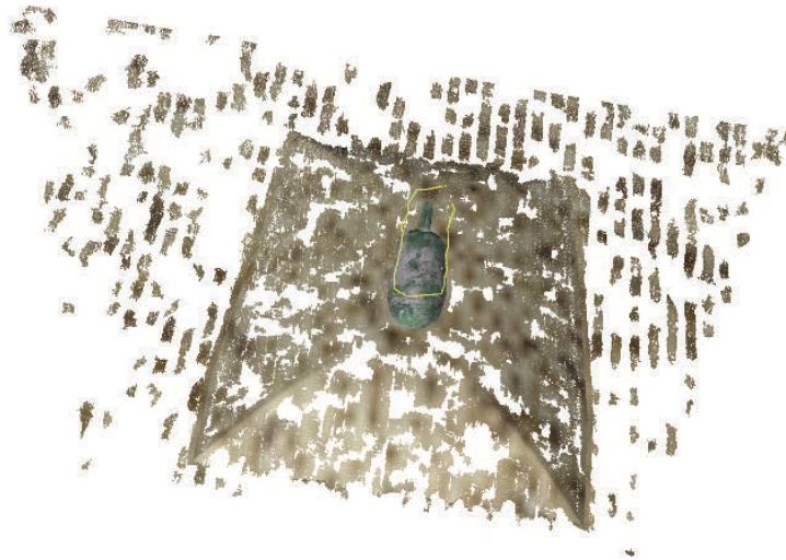
Fig. 2: Corresponding path generated (yellow line) from the 3D point cloud using projection and concave hull methods.
