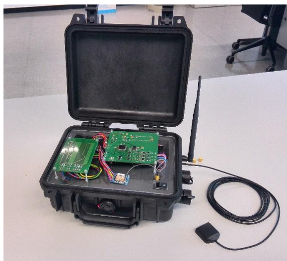
Figure 1 Volcanic seismic acquisition equipment
