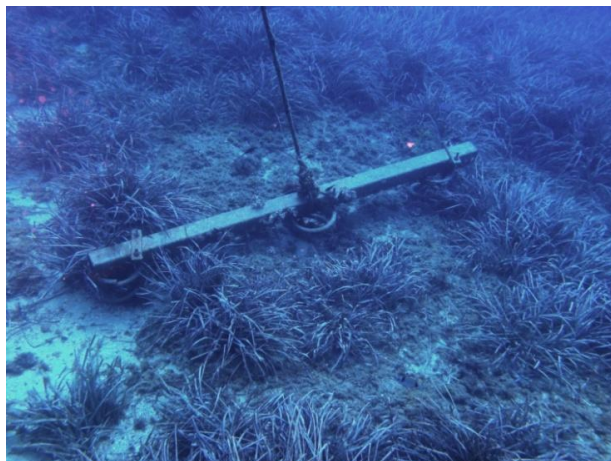
Fig. 1. Anchorage system into Posidonia oceanica seabed.
