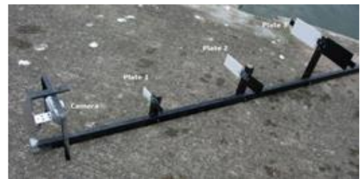
Fig. 1: Secchi 3000 Device. The pole weights 1.7kg + the camera, total length is 1.56m.
