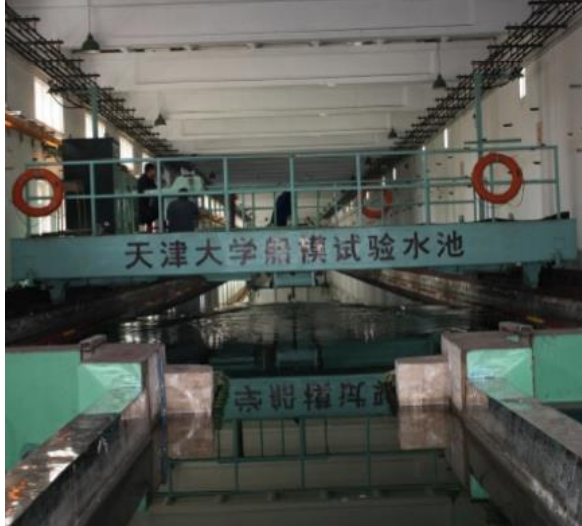
Fig. 3. Example of a tow tank facility with the trolley towing an instrument at accurate speed in the middle of the tank.
