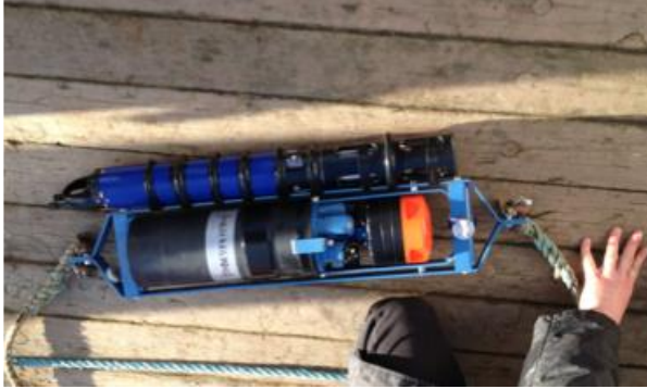
Fig. 10: One Seaguard (Aanderaa) and one EXO2 (YSI) deployed back to back during 2012-2013. The two instruments are carrying the following sensors: Cond/Sal (2), Temp (6), Pressure (2), Wave/Tide, O 2 (2), pCO 2 (2), FDOM, ChlA-Blue green-Total algae, pH/ORP and Currents (speed and direction). Copper coverage and a wiper provide Antifouling.
