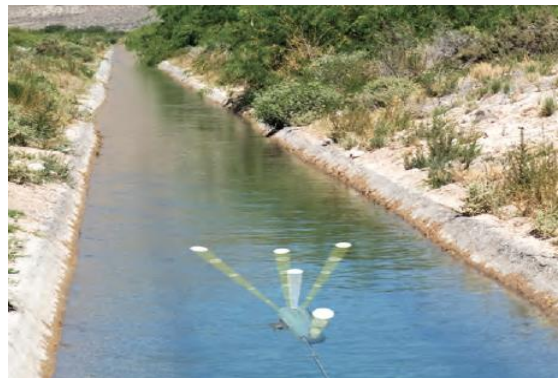
Fig 1. Sontek IQ compact acoustic doppler profiler installed in an irrigation canal to monitor flow.
