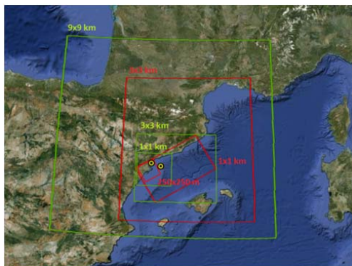
Fig.4. Schematization of the domains for the simulation. In green the boundaries for the meteo model, in red for the wave/current models. The outer boundary conditions come from a full Western Mediterranean model not shown in the figure.
