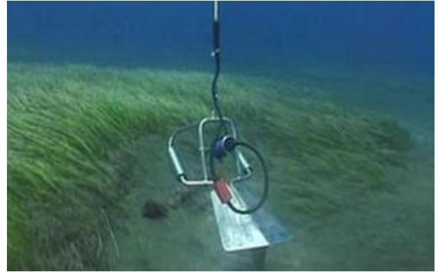
Fig. 1. Underwater skate equipped with the XeoTV system, used to record the status of the seafloor.
