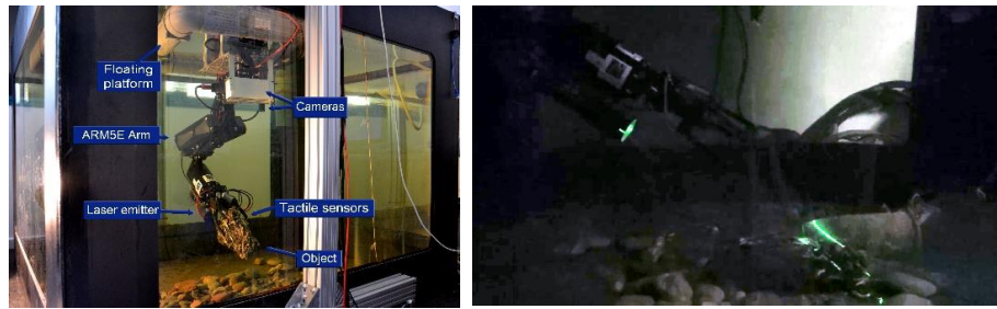
Fig. 1 The vehicle is equipped with a light-weight robot arm and a 4-finger gripper, an underwater looking down camera and the 3D laser stripe emitter (left). The laser stripe emitter attached to the arm, scanning the floor (right).
