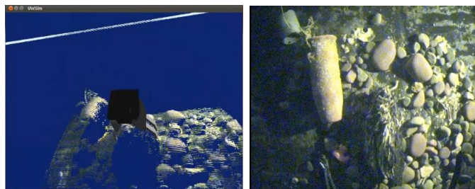
Fig. 2 Reconstructed scenario in the UWSim underwater simulator: 3D point cloud and CAD model of the end-effector (left). Real scenario captured by the camera with the two experimental objects (right).
