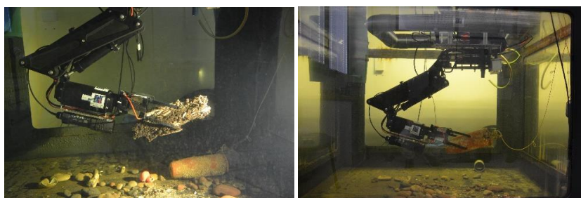
Fig. 3. The I-AUV grasping a wooden trunk (left) and an amphora (right) inside the water tank
