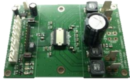
Fig. 5 DRV8432 dual full bridge driver for the two lateral thrusters
