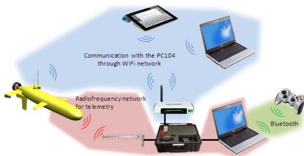
Fig. 3 Diagram for communication system of Guanay II AUV
