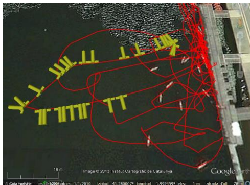
Fig. 9 Tests at Canal Olímpic de Catalunya in Castelldefels for test the thrusters control system and the communications with the vehicle
