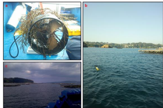
Fig 2.- Operational risks. Top left (a) Seaweed obstructing the propeller. Bottom left (c), Mussel farm. Right (b), AUV close to a mussel raft. (Sea Technology, August 2012.)
