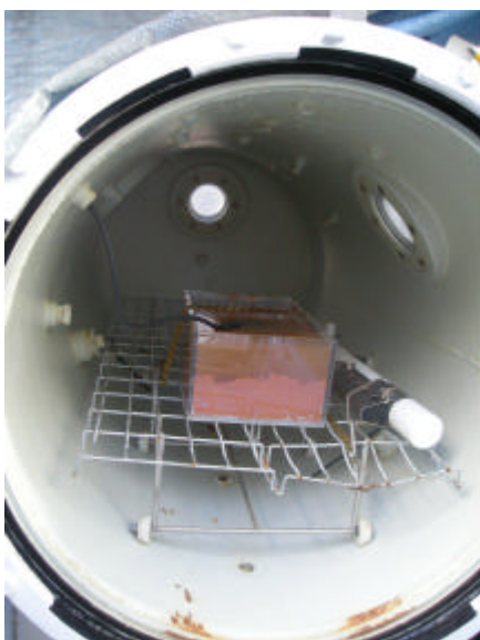
Fig.10 Sediment box and geophone inside the hyperbaric chamber
