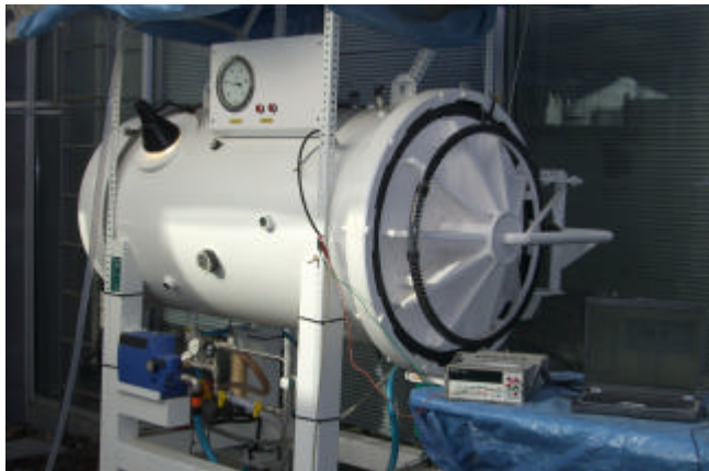
Fig. 8 Sediment box and geophone inside the hyperbaric chamber
