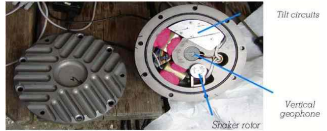
Fig 10. Internal arrangement of CARRACK geophone modified with shaker motor (base view shown).
