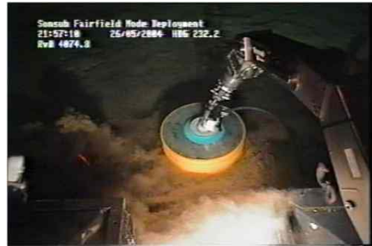
Fig 3. ROV deployment of seismic node in deep water
