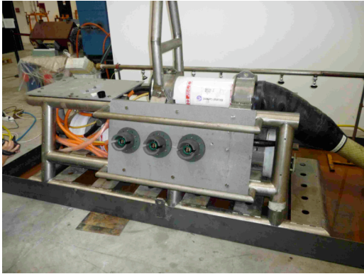
Fig. 2. Frame Termination Assembly ready to be deployed
