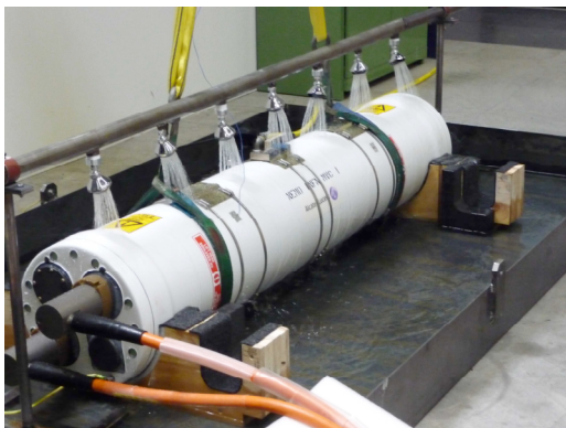
Fig. 4. Medium Voltage Converter under test
