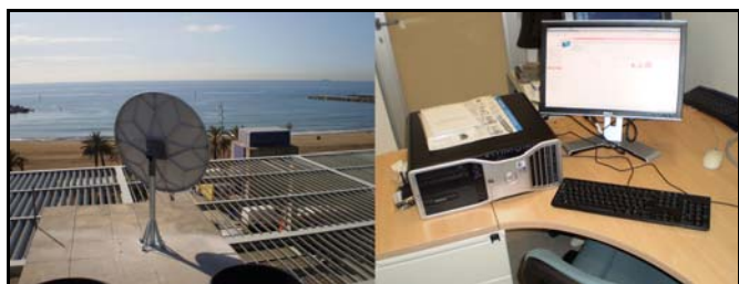
Fig. 3. EUMETCast receiving system
