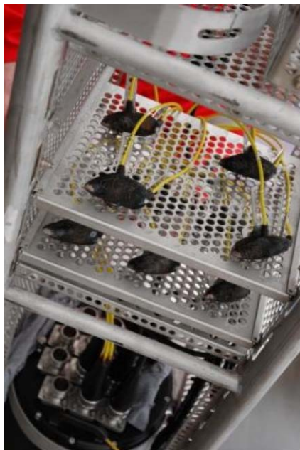
Figure 3: The Biotaguard system ( http://www.biotaguard.no/visartikkel.asp?id=586 ) combines biological (mussels), physical and chemical sensors into a powerful assembly for environmental monitoring.
