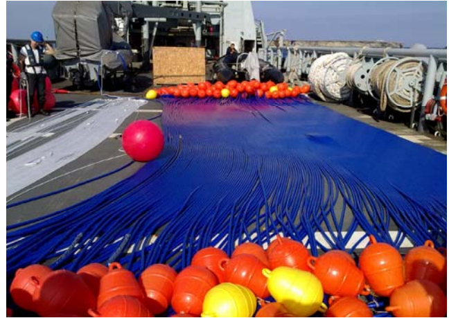
Fig. 6. Stern of the "Mar Caribe" patrol boat, of the Spanish navy, with the cable ready for the deployment and the guide to drive the cable toward the Alborán island.
