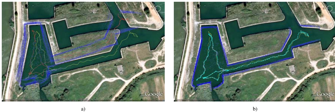
Fig. 2. Results: a) Trajectory and map generated with odometry (red). DGPS trajectory (yellow) used as a ground truth. b) Map and trajectory (dotted cyan) generated with the SLAM algorithm.
