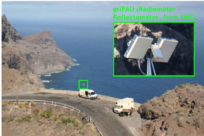
Fig. 5. griPAU deployed during the ALBATROSS 2009 field experiment.
