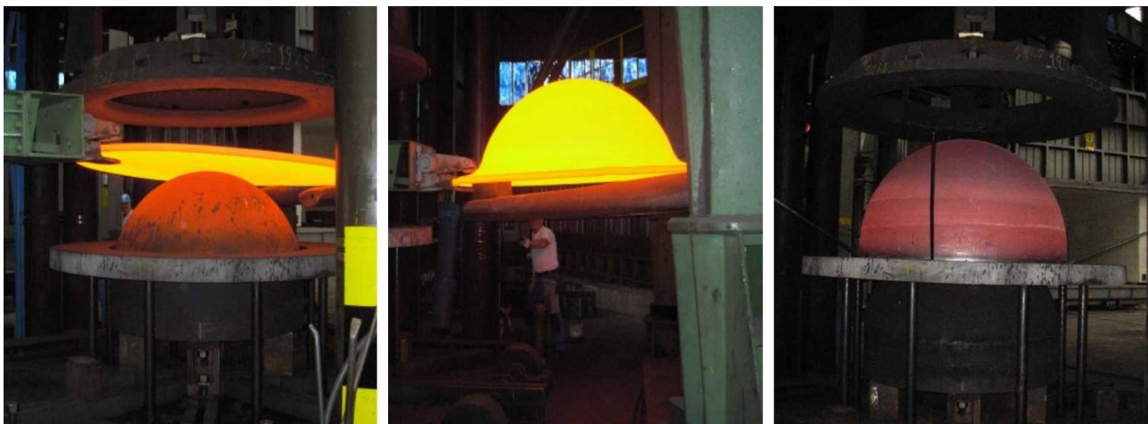
Fig. 2. Deep drawing of one hemispherical dished head of Ictineu 3 pressure hull (courtesy of ATB Riva Calzoni S.p.A.)
