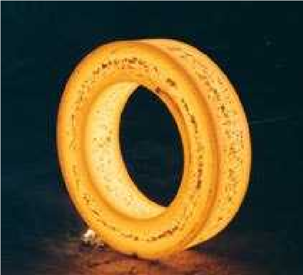
Fig. 3. Forged ring before heat treatment (courtesy of Special Flanges S.p.A.)
