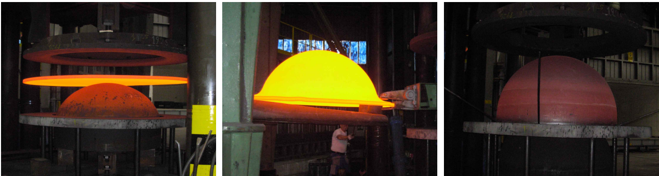
Deep drawing process of one of the hemispheres of the pressure hull
