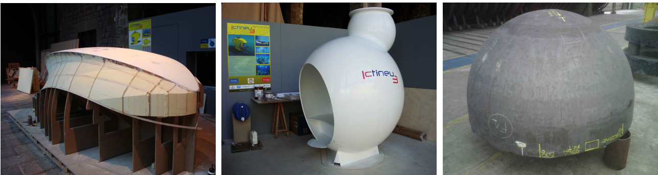
Exterior hull model. 1:1 scale model of the pressure hull. One of the built four stainless steel hemispheres of the pressure hull.
