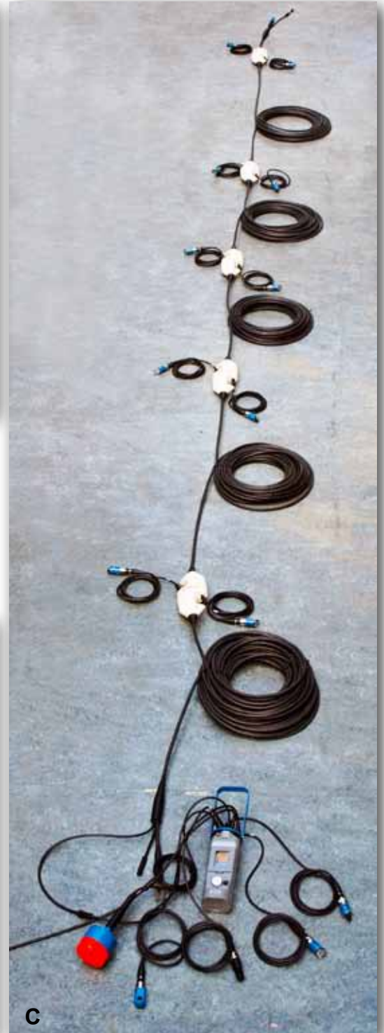
Figure 3. Aanderaa Data Instruments Seaguard sensor system designed for UNC-Chapel Hill's coral reef project. A, Seaguard base unit with current meter, optode O 2 sensor, CTD and turbidity sensors. B, wet mateable Optode sensors on 3 meter length fly leads. C, 170 meter optode sensor string with Seaguard base unit, .
