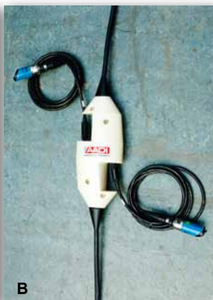
Figure 3. Aanderaa Data Instruments Seaguard sensor system designed for UNC-Chapel Hill's coral reef project. A, Seaguard base unit with current meter, optode O 2 sensor, CTD and turbidity sensors. B, wet mateable Optode sensors on 3 meter length fly leads. C, 170 meter optode sensor string with Seaguard base unit, .
