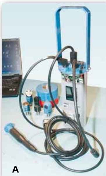
Figure 3. Aanderaa Data Instruments Seaguard sensor system designed for UNC-Chapel Hill's coral reef project. A, Seaguard base unit with current meter, optode O 2 sensor, CTD and turbidity sensors. B, wet mateable Optode sensors on 3 meter length fly leads. C, 170 meter optode sensor string with Seaguard base unit, .
