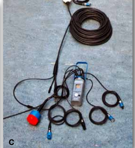
Figure 3. Aanderaa Data Instruments Seaguard sensor system designed for UNC-Chapel Hill's coral reef project. A, Seaguard base unit with current meter, optode O 2 sensor, CTD and turbidity sensors. B, wet mateable Optode sensors on 3 meter length fly leads. C, 170 meter optode sensor string with Seaguard base unit, .
