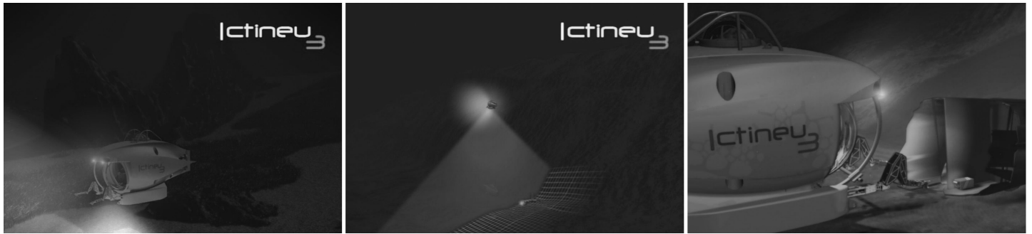
Fig.1: Ictineu 3 possible missions, from left to right: archaeological photo-mosaic, fine scale bathymetric surveying, and black box recovery.
