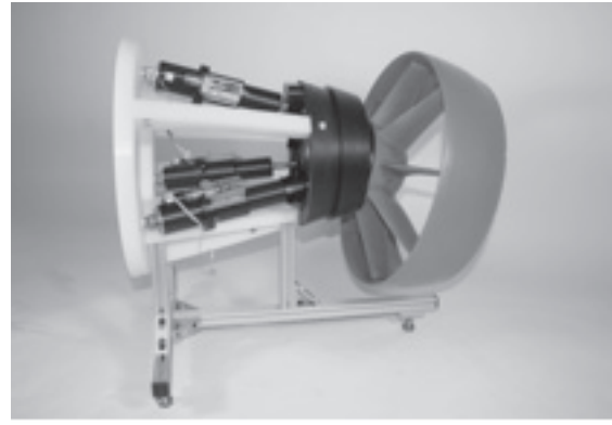
Figure 4: External comparison of the Gimbaled Tailcone and the False Center Tailcone
